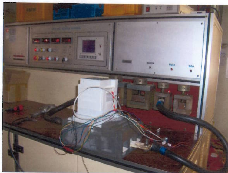
Photo. 4. overload release test; single phase
