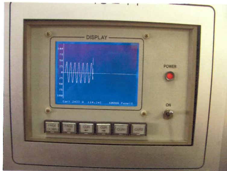
Photo. 5. oscilogram of the overload release test
