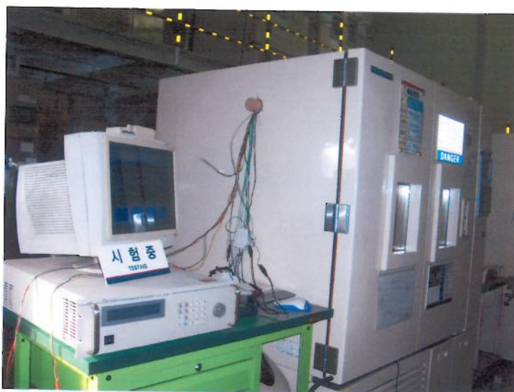
Photo. 1. test arrangement of outer chamber - Programmable power source and temperature chamber
